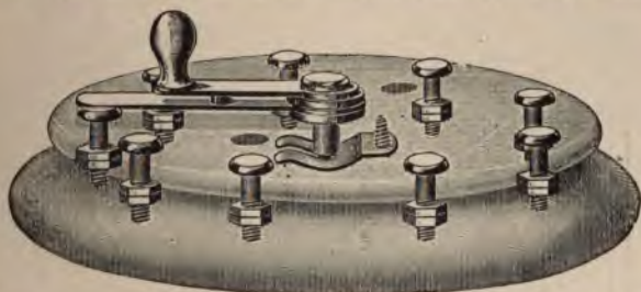
FIG. 188.—Diagram of the construction of a form of button contact switch. The common wire and home apparatus line are wired to the lever, the others, to the binding nuts on the circumference.
